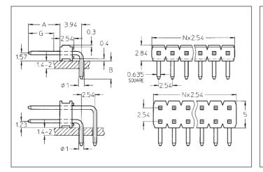
Series 890/892 square pin headers are cost efficient thanks to selective gold plating on pins made of copper alloy
