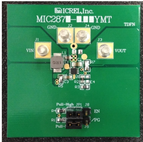
Figure 1. MIC2875-AYMT Evaluation Board
