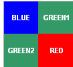
Figure 6. Color Filter Arrangement on the Pixels
