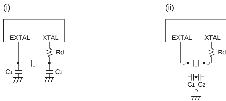
Fig. 13. Recommended Oscillation circuit
