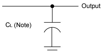
Note:  $C_L$  includes probe and jig capacitance.
