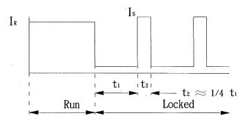
3rd wire signal Run : Square Wave Locked : VH or VL
