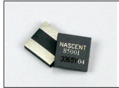
NASCENTechnology, Inc. has developed a series of high temperature, RoHS compliant inductors using low temperature co-fired ceramic (LTCC) ferrite usable to 300°C that feature low profile, rugged packaging, and self shielding characteristics. Part mass 0.6 to 1.2 g
