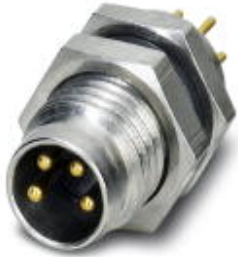
Sensor/actuator flush-type connector, male, 4-pos., M8, rear/screw mounting with M8 thread, with straight solder connection
