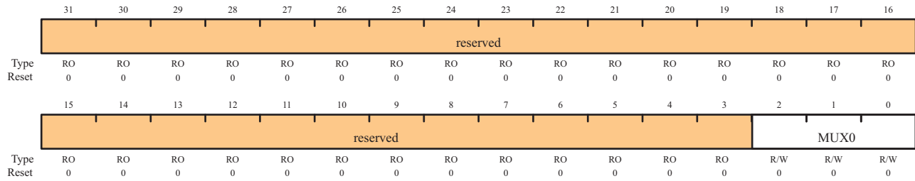
ADC Sample Sequence Input Multiplexer Select 3 (ADCSSMUX3)
