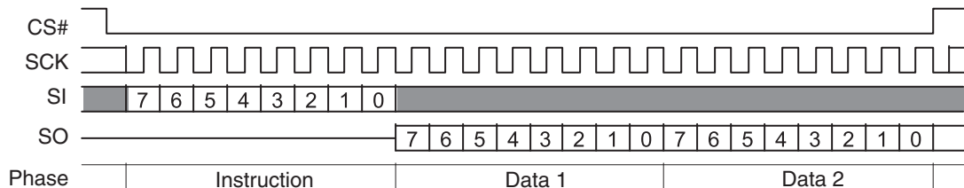
Figure 9. Single Bit Wide I/O Command without Latency
