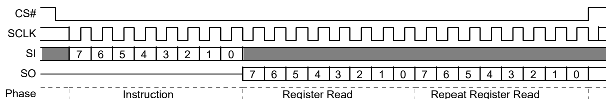
Figure 52. Read Configuration Register (RDCR) Command Sequence
