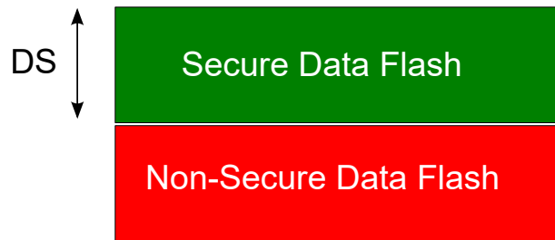
Figure 13-3. SAM L11 Data Flash Memory Mapping
