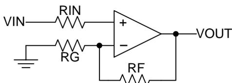
Figure 17. Operational Amplifier Schematic for Noninverting Configuration
