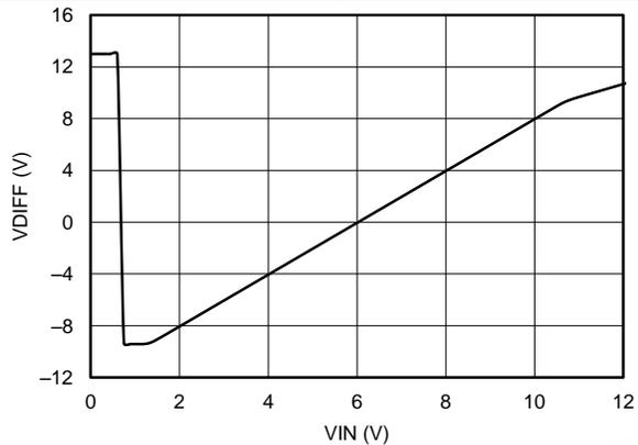
Figure 14. Differential Output Voltage vs Input Voltage
