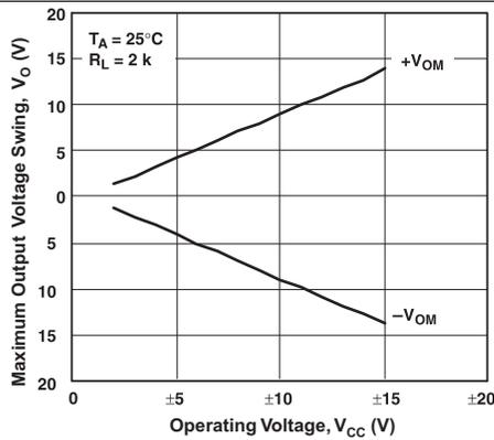
Figure 9. Maximum Output Voltage Swing vs Operating Voltage
