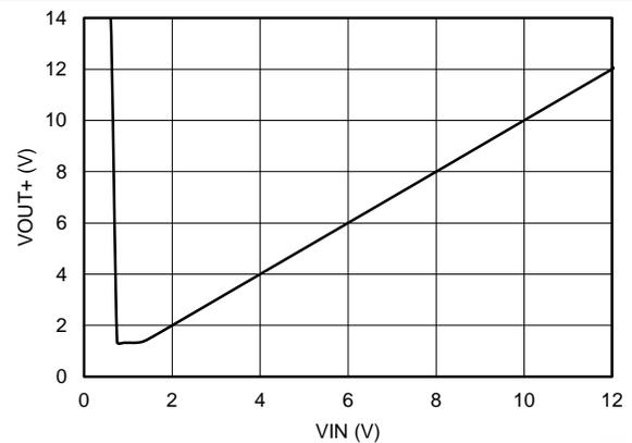
Figure 15. Positive Output Voltage vs Input Voltage
