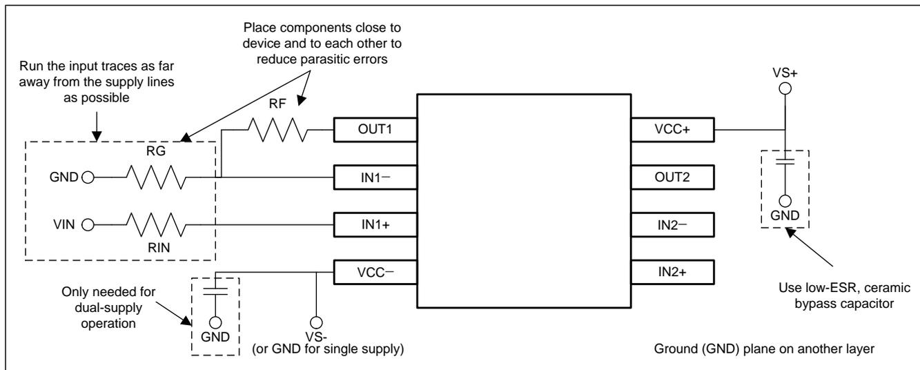
Figure 18. Operational Amplifier Board Layout for Noninverting Configuration
