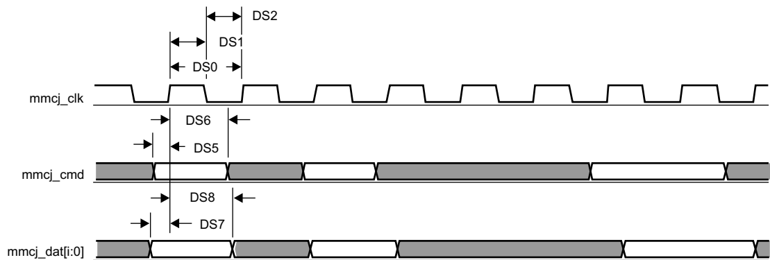
图 7-81. MMC/SD/SDIOj in - Default Speed - Receiver Mode
