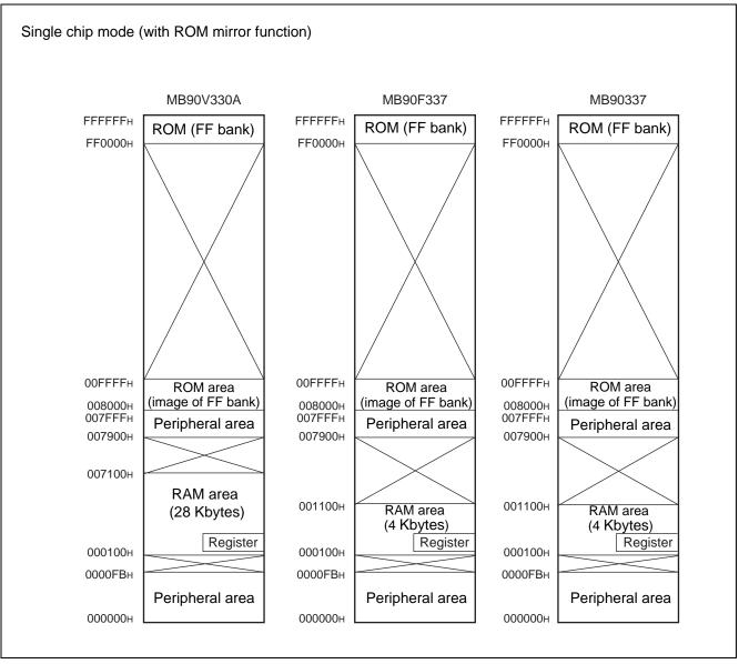
Notes: • When the ROM mirror function register has been set, the mirror image data at higher addresses ("FF8000H to FFFFFFH") of bank FF is visible from the higher addresses ("008000H to 00FFFFH") of bank 00.
