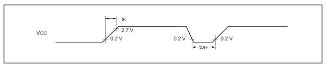
Note: Sudden change of power supply voltage may activate the power-on reset function.
