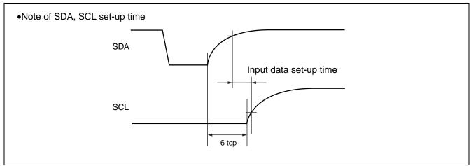
Note: The rating of the input data set-up time in the device connected to the bus cannot be satisfied depending on the load capacitance or pull-up resistor.
