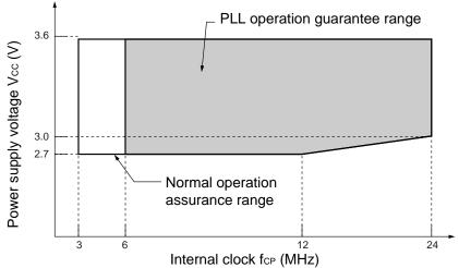
Note: When the USB is used, operation is guaranteed at voltages between 3.0 V to 3.6 V.
