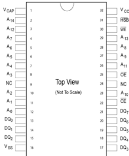
Figure 1. Pin Diagram: 32-Pin DIP
