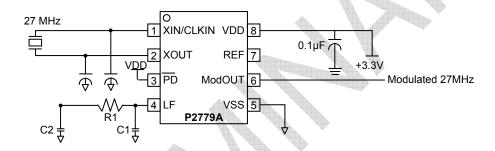
PD selection: Power dissipation can be reduced by completely turning off the IC.
