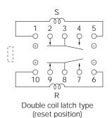
S: Coil polarity of set (operate) R: Coil polarity of reset (release)
