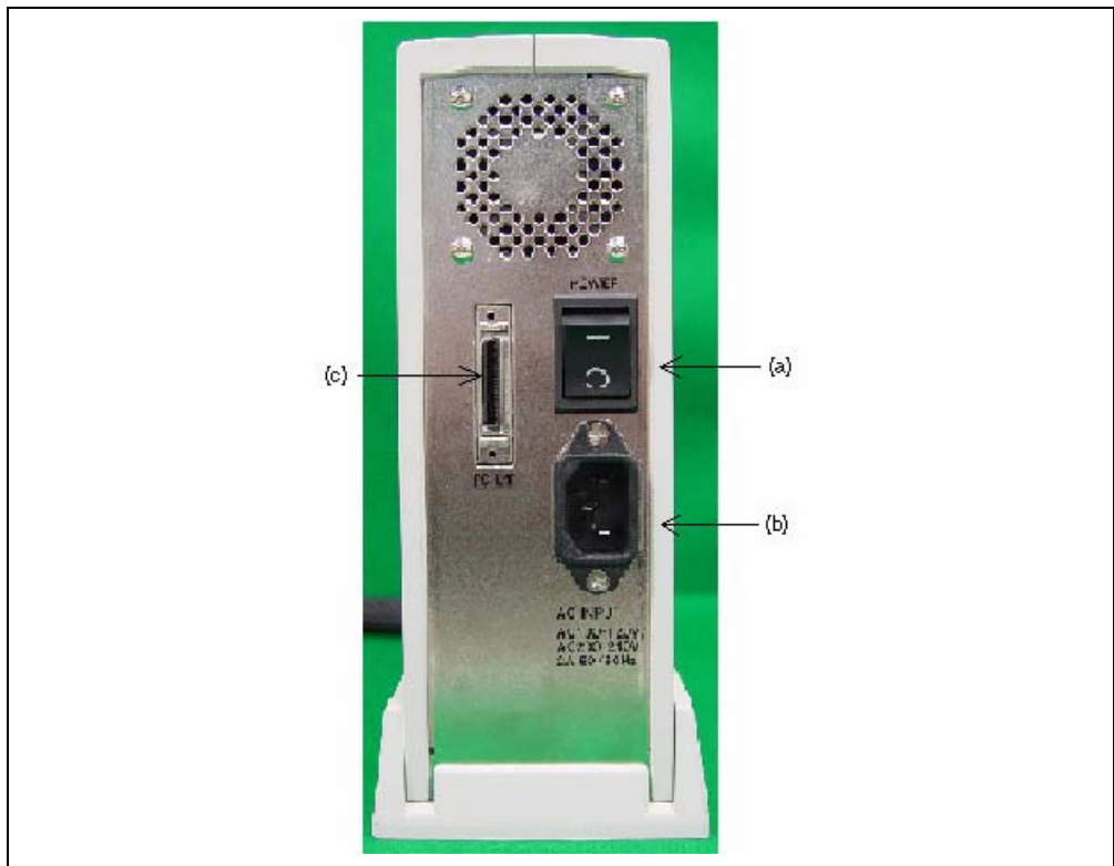
Figure 1.3 E6000H Station: Rear Panel
