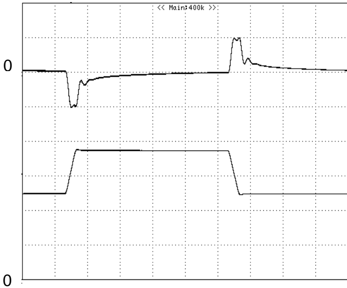
Figure 8: Output voltage response to step-change in load current (75%-50%-75% of I_o , max; di/dt = 0.1A/\mu s ). Load cap: 10\mu F tantalum capacitor and 1\mu F ceramic capacitor. Top Trace: V_{out} (50mV/div, 200us/div), Bottom Trace: I_{out} (5A/div). Scope measurement should be made using a BNC cable (length shorter than 20 inches). Position the load between 51 mm to 76 mm (2 inches to 3 inches) from the module
