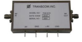
The TA024-025-35-35 is a PCB based 4 W power amplifier designed for operation in the 2.4 to 2.5 GHz frequency range. This amplifier utilizes high power devices that provide excellent linearity and high gain. High efficiency operation is achieved by using hybrid MIC designs and advanced GaAs PHEMT devices. The amplifier requires a +8V DC power supply and a -2V DC power supply.
