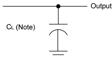
Note: CL includes probe and jig capacitance.
