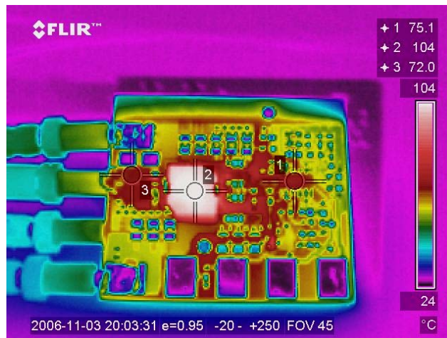
Figure 11a – Temperature Distribution, Top side
