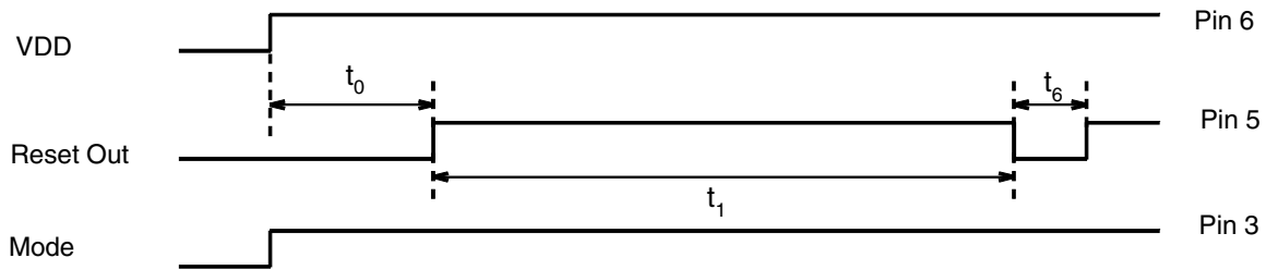
Figure 4. Power-on Reset and Switch-over Mode
