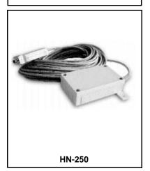
The HN-250 is a versatile, low cost, multi-purpose 2.4 GHz frequency-hopping wireless data modem. Built around the WIT2450 radio, the HN-250 has an integral 6dB patch antenna creating a "single piece" modem. Communication with the HN-250 is through a 921.6kbps (USB version only) or 115.2Kbps (USB or RS-232 versions) asynchronous serial port supporting a standard RS-232 interface. The HN-250 communicates over the air at 1.23Mbps and supports both point-to-point and point-to-multipoint networks.
