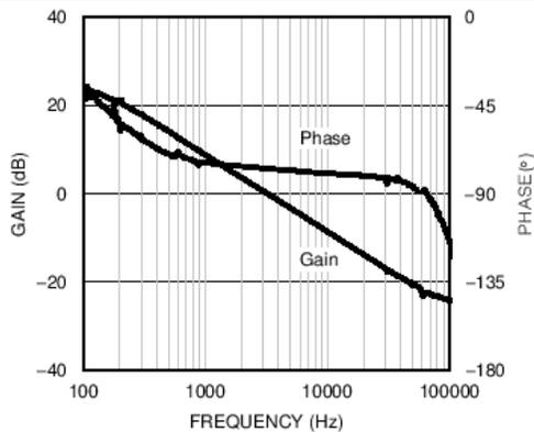
**Figure 21. Modulator Gain and Phase - Buck Mode**
