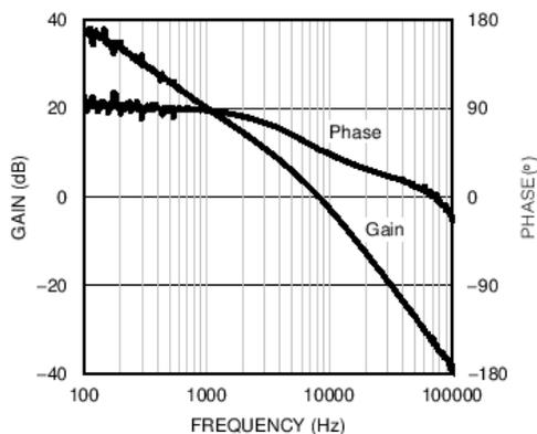
**Figure 25. Overall Loop Gain and Phase - Buck Mode**
