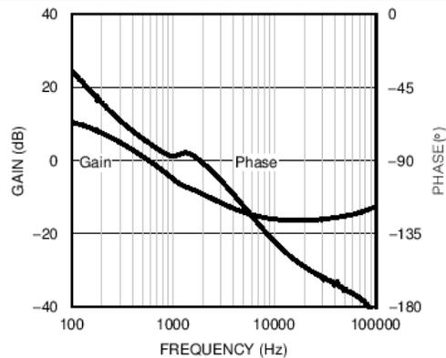
**Figure 22. Modulator Gain and Phase - Buck-Boost Mode**
