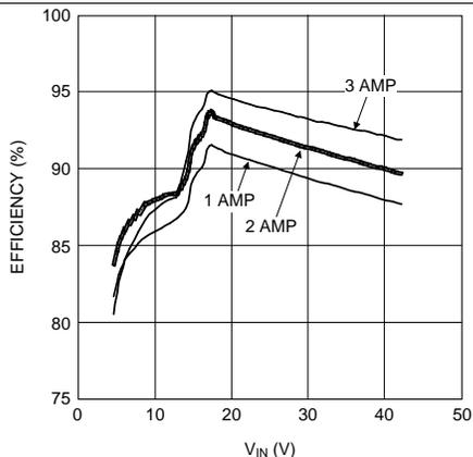
Figure 1. Efficiency vs VIN and IOUT VOUT = 12 V
