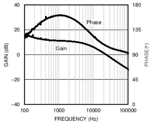
**Figure 24. Error Amplifier Gain and Phase - Buck-Boost Mode**
