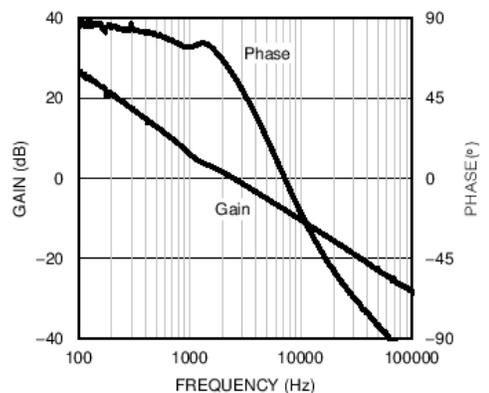
**Figure 26. Overall Loop Gain and Phase - Buck-Boost Mode**
