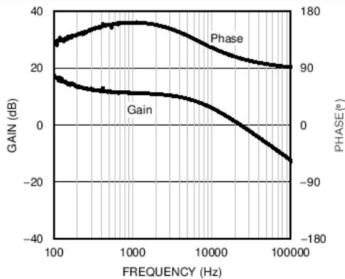
**Figure 23. Error Amplifier Gain and Phase - Buck Mode**
