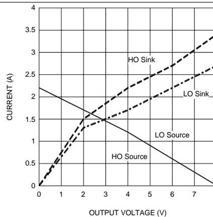
Figure 6. LO and HO Peak Gate Current vs Output Voltage VCC = 8 V
