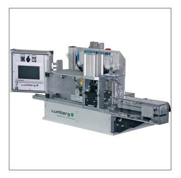
Semiautomatic harnessing machine for termination of RAST 2.5 connectors in insulation displacement technology, larger base machine, with integrated station for keying cutting, individual upgrading possible
