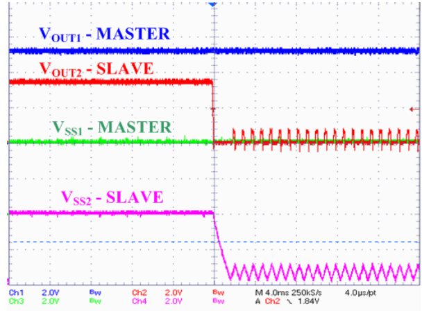
Figure 64. Master Voltage – End of Augmented OLM
