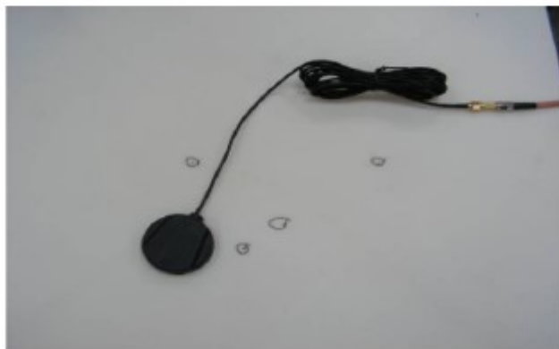
Wi-Fi antenna test with plastic
