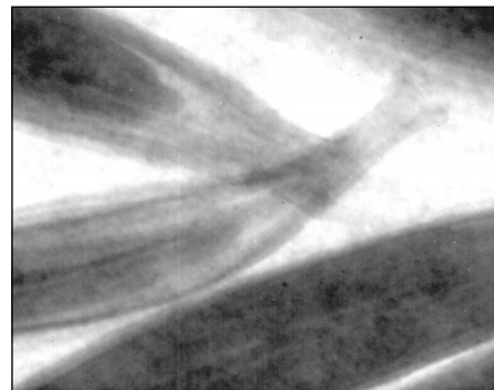
▲Seeds X-ray tube voltage: 25 kV Geometrical magnification rate: \times 2.1
