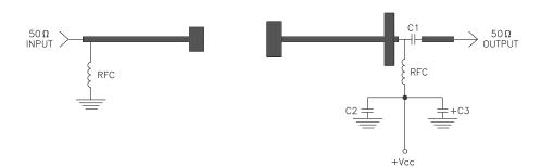
= Microstrip on 0.020" Teflon Fiberglass, Er=2.55 C1,C2 = ATC 'A' 47pf C3 = 10 Mfd @ 35 Volts
