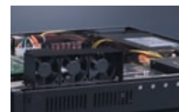
Three filtered 10-CFM cooling fans are on the front
