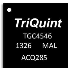
28-pin 5x5mm QFN package
