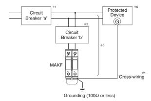
\*1. The circuit breaker must be installed.
