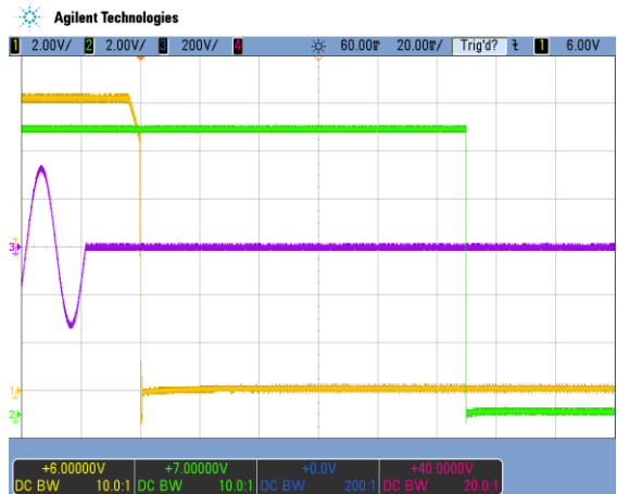
Figure 10 - Turn-Off AC Line 230 VAC, full load (20 ms/div) CH1: V1 (2 V/div); CH2: VSB (2 V/div); CH3: Vin (200 V/div)
