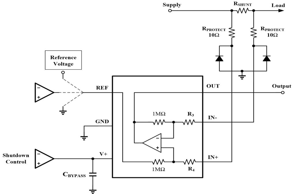
**Figure 5. WS74199 Transient Protection Using Dual Zener Diodes**
