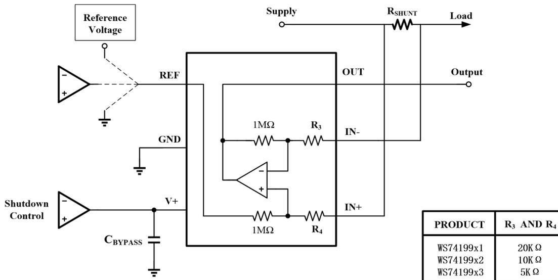
NOTE: 1-MΩ paths from shunt inputs to reference and the WS74199 outputs.
