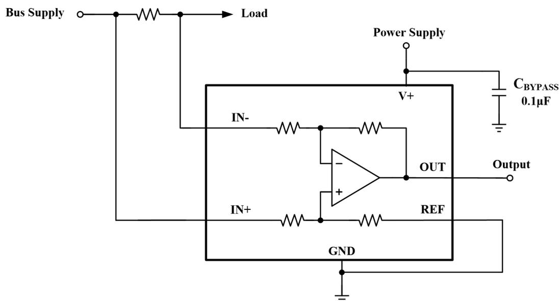
**Figure 8. Unidirectional Application Schematic**
