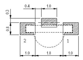
Note: Tolerances unless mentioned ±0.1mm. Unit = mm Suggested pad dimension is just for reference only. Please modify the pad dimension based on individual need.
