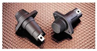
Panel mount fuseholders are available for supplementary or Class CC branch circuit protection. Class CC fuses have a rejection feature on one end cap which mates with the rejection feature of Littelfuse Class CC fuse blocks and fuseholders to prevent the installation of fuses with lower voltage ratings or interrupting ratings. Watertight version must be front panel mounted.
