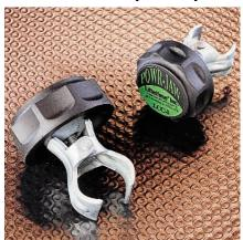
POWR-JAW clamps improve the contact between fuse and clip. The unnecessary heat from poor contact due to the loss of spring force in the clips can cause nuisance fuse opening and premature aging of surrounding components.
