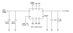
TV Series Clipped Sinewave Test Circuit
