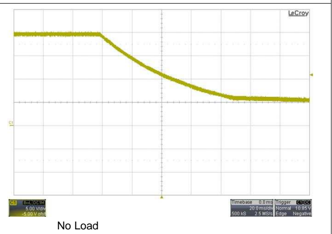
Figure 55. VBUS 20 V – 5 V Transition
