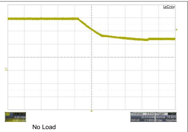
Figure 53. VBUS 20 V – 12 V Transition
