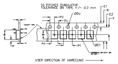
REEL DIMENSIONS 10.0 А inches 7.0 13.0 177.8 254.0 330.2 mm в inches 2.50 4.00 3.75 mm 63.5 101.6 95.3 Таре Width С mm 13.0 +0.5 / -0.2 D mm 16.4 16.4 16.4 16.0 +2.0 +2.0 -0.0 +2.0
