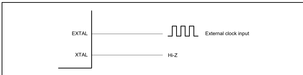
Figure 9.5 Equivalent circuit for external clock
