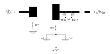
= Microstrip on 0.0186" Teflon Fiberglass, Er=2.55 C1 = ATC 68pF B-CASE C2 = ATC 68pF A-CASE C3 = 1.0 MFD 35V RFC = 4 turns #22 wire 1/16" I.D.
