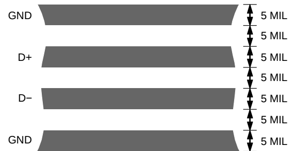
Figure 12. Typical Assignment of Signal Tracks
