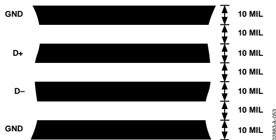
Figure 54. Arrangement of Signal Tracks
