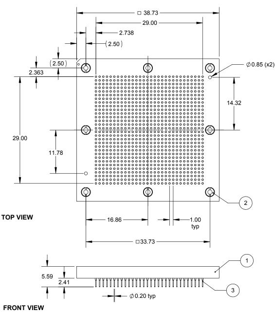
\*Note: BGA pattern is not symmetrical with respect to the mounting holes. It is shifted 0.375 to the right of center.
