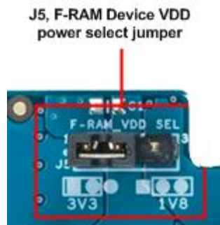
Figure 1. F-RAM Device VDD (F-RAM_VDD) Selection Jumper
