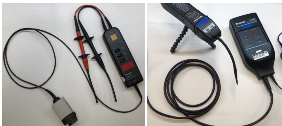
Figure 14. Probe Examples, (a) Tektronix® Differential Probe THDP0200 (150 V Range), (b) Tektronix® IsoVu® TIVH05 Probe (TIVPMX10X, ±25 V Sensor Tip)
