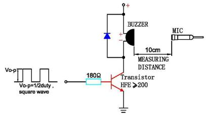
In the measuring test, buzzer is placed as follows:
