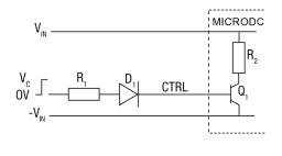
$D_1$  (eg 1N4001) is required to provide high impedence when the signal is low. From the WRA-YLS-3W specification, the drive current to operate this
