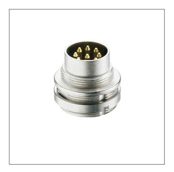
Chassis plug acc. to AISG specification and IEC 61076-2-106, IP 68, with threaded joint and solder terminals, for front mounting
